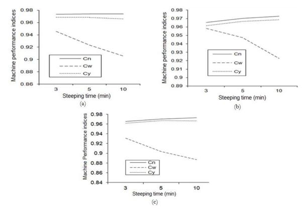
Figure 6. Effect of steeping time on the coefficients of dehulling, coefficient of wholeness and yield for three varieties of cowpea using the inclined beaters at 10 s resident time ((a) = Red drum, (b) = White drum, (c) = Ife brown,  $C_n$  = coefficients of dehulling,  $C_w$  = coefficients of wholeness and  $C_y$  = coefficients of yield))
