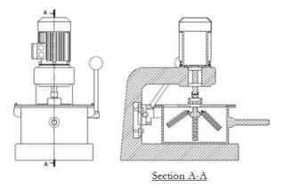
Figure 2b. Sectional view of the cowpea dehuller showing the details of inclined beaters
