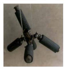
Figure 5a. The rubber-lined inclined beaters
