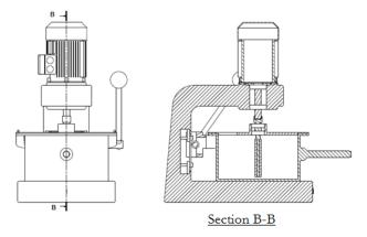
Figure 3b. Sectional view of the cowpea dehuller showing the details of vertical beaters
