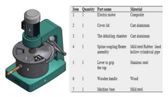
Figure 4. Isometric drawing of the experimental machine showing machine parts
