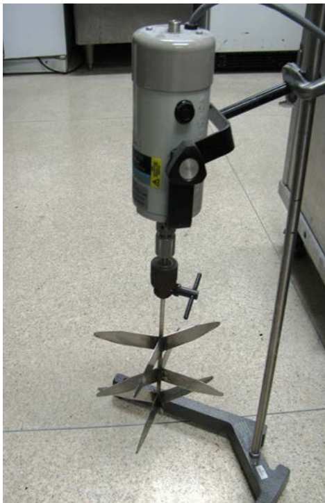
Figure 1. Modified servodyne mixer used to wash wheat bran
