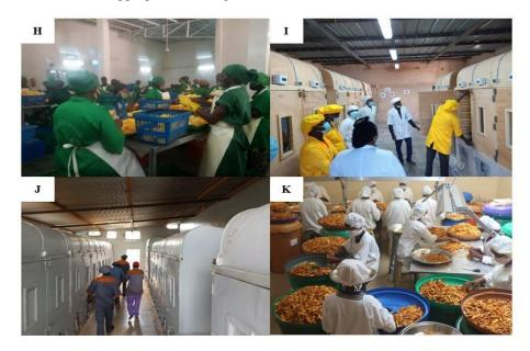
Figure 4. Appropriate staff attire (Legend: H: Pulping and cutting; I: Enclosing of cut mangoes; J: Dryer control (temperature, drying level, functionality); K: Sorting and classification of dried mangoes)
