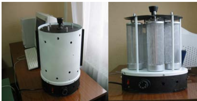
Figure 1. Infrared, ecological, universal, portable dryer based on indirect application of electricity as the heat source
