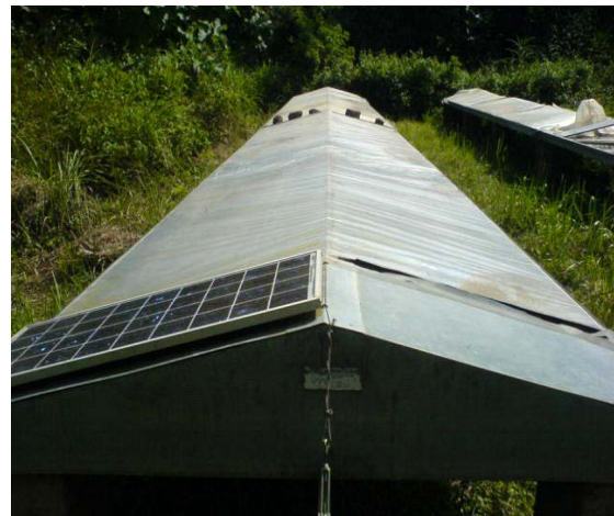
Figure 2. The pictorial view of new designed solar tunnel dryer
