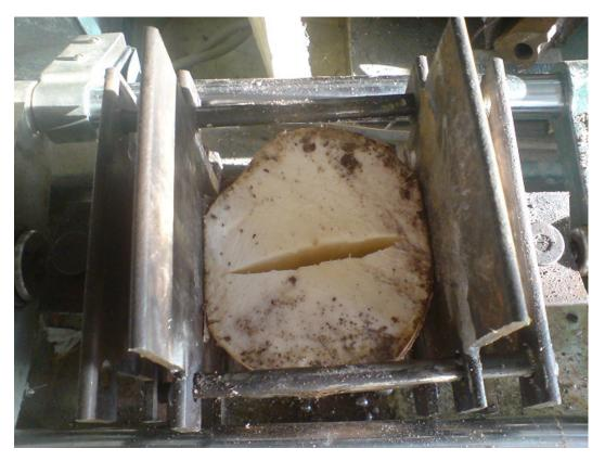
Figure 2. The point of breakage of a certain tuber slice
