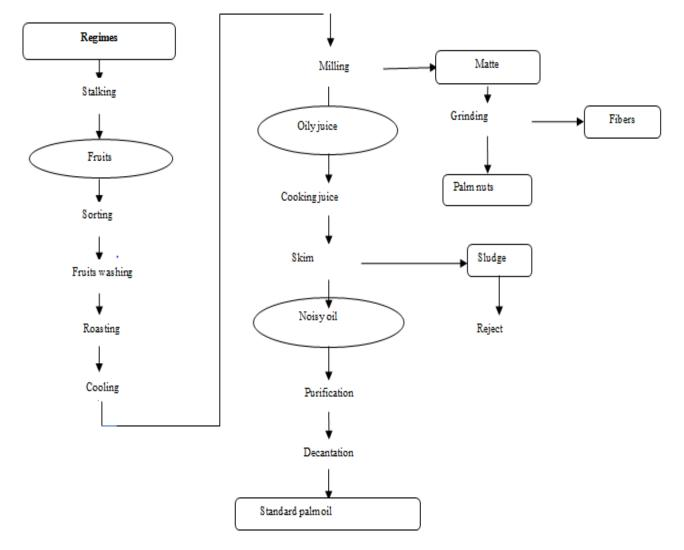
Figure 4. Artisanal process for producing standard palm oil [9]
