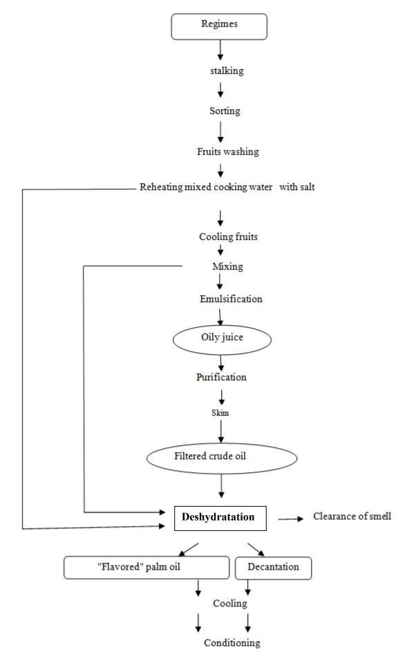
Figure 5. Artisanal process for producing of "flavored" palm oil [11]
