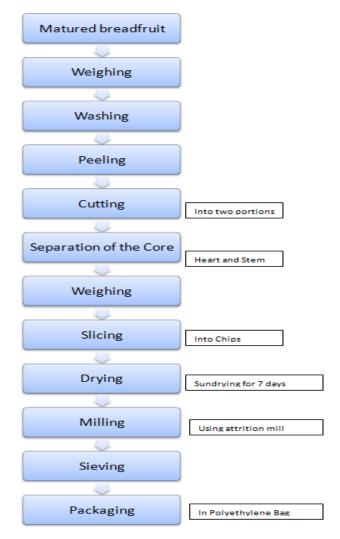
Figure 1. Process flow diagram for Breadfruit flour (Source: Akubor PI., et al (2000)) [22]
