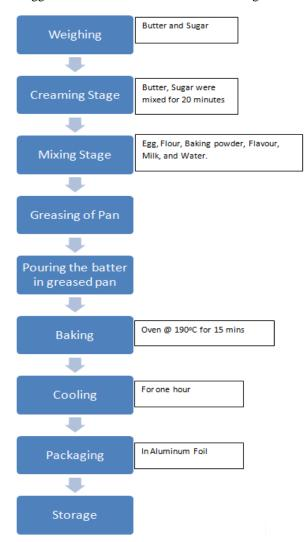
Figure 2. Process flow diagram for production of Cake (Source: [23])
