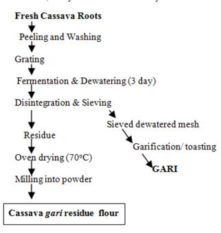
**Figure 1.** Flow chart for production of cassava residue flour obtained from *gari* processing operation. Source: [16]
