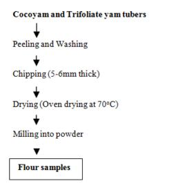
**Figure 2.** Flow chart for the production of cocoyamflour and trifoliate flour. Source: [17]
