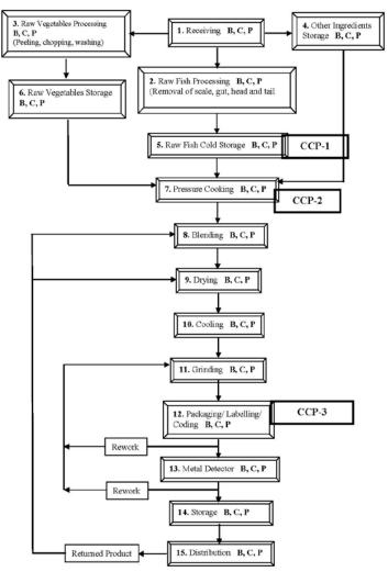
Figure 1. Description of Process Flow Diagram
