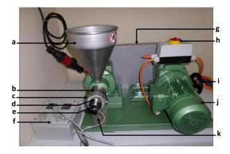
**Figure 2.** Komet press (CA 59 G, IBG Monforts Oekotec, Mönchengladbach, Germany) coupled to a heating system: a: feed hopper; b: perforated cylinder; c: strip heater; d: screw head; e: outlet nozzle of presscake; f: thermoregulator; g: gear transmission; h: start button; i: gearbox; j: moter; k: oil collection container
