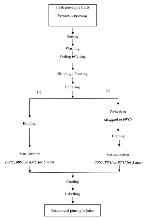
Figure 1. Flow chart for the production of 6 categories of pasteurized pineapple juice
